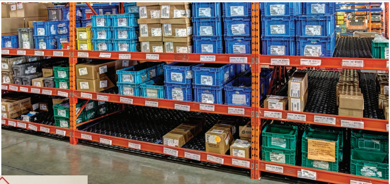
▲ Multi-level Carton Flow showing full width bed using plastic wheels
