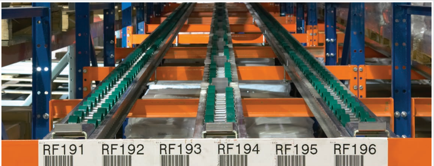
▲ Heavy duty deep lane pallet flow with wheels in three double row configurations
