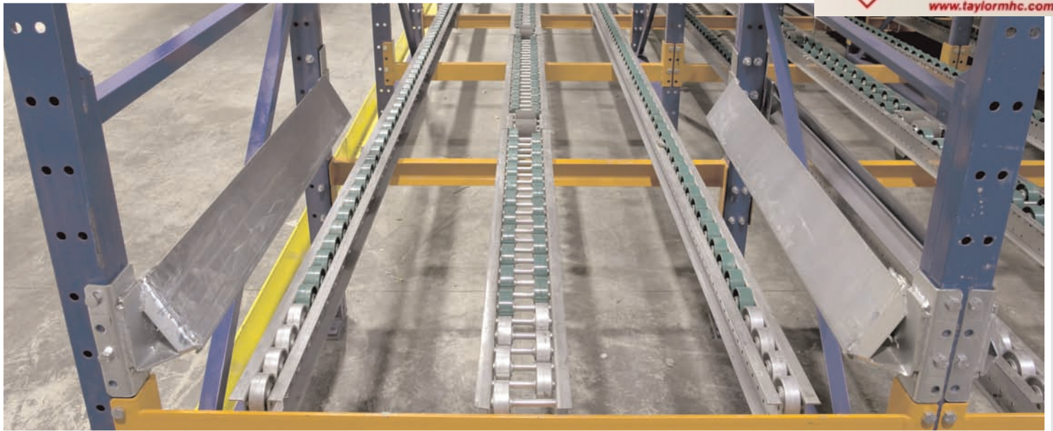
▲ Deep lane pallet flow with wheels in a single-double-single configuration for standard GMA/CHEP pallets
