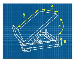
For applications utilizing small or shallow containers that do not require vertical repositioning, the Fixed Height Tilter is the ideal choice. Available in 2000 Lbs. and 4000 Lbs. They can be mounted on the floor or a fixed height table top.
