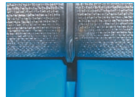
V-guided belt and the v-guided frame
