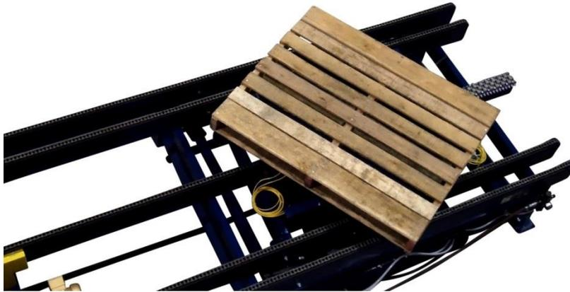
Using a strong design incorporating flat side bar chain, Nylatron wear strips and a heavy duty lift and rotate turning plate, Alba provided a unit that met the requirements and would last for years to come. For more
