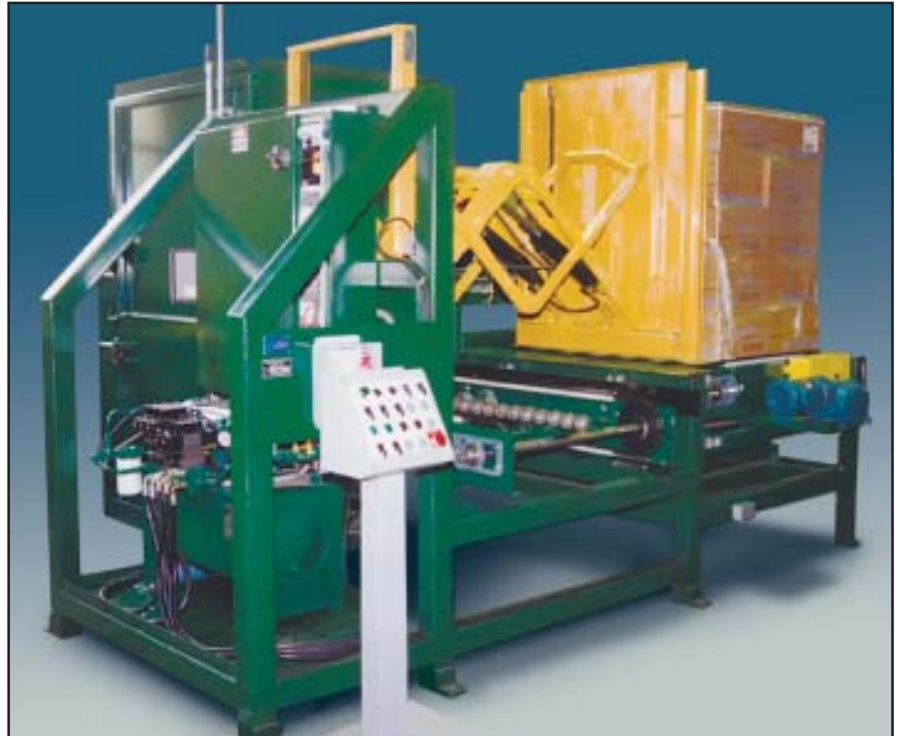
RM-1000 Transfers Cased Product from Pallet to Slip Sheet
