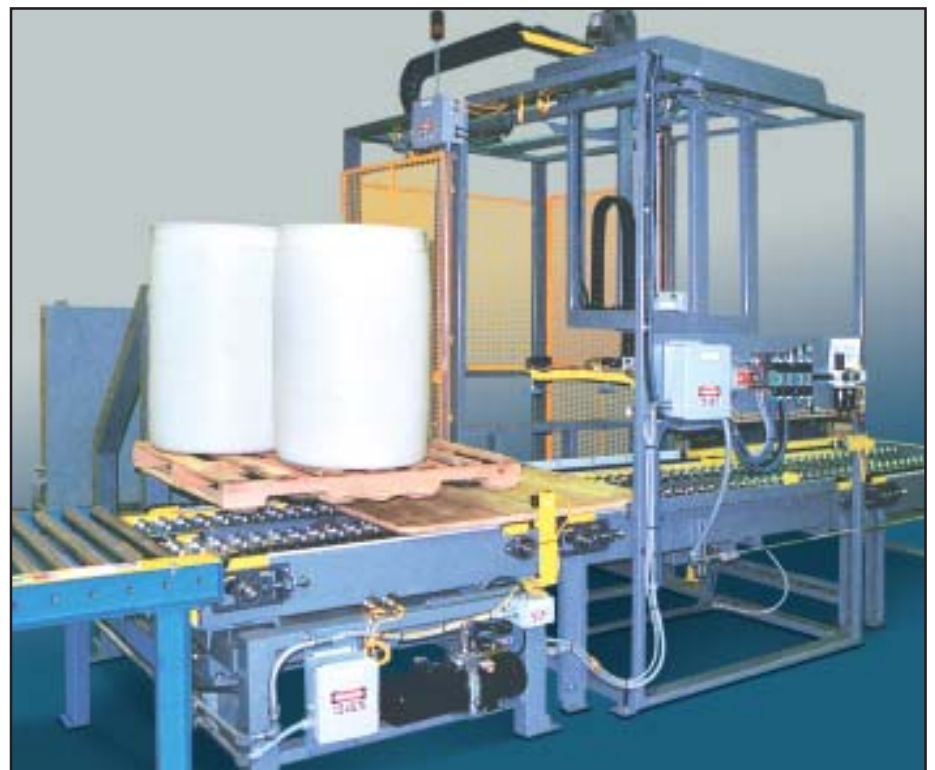
Palletized product is lifted from captive pallet and conveyed into a pallet stacker
