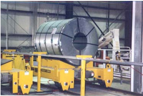
Fully automated electric powered coil car.
