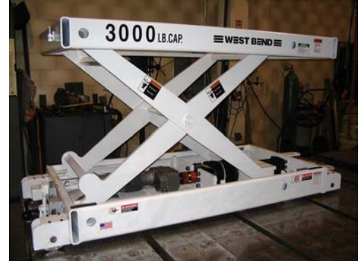
3,000 pound capacity electric screw powered mobile lift table.
