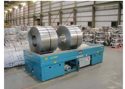
50 ton capacity propane engine powered transfer car.
