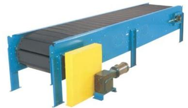
Slat Conveyors are commonly used in assembly line operations where product moves at a slow rate of speed through several operator workstations. The slats are made of formed 7-gauge steel, 5-7/8" wide x 1-1/2" deep on 6" centers. The strength of the individual slats is ideally suited to convey larger and heavier products like washing machines, furniture, and larger automobile parts.
