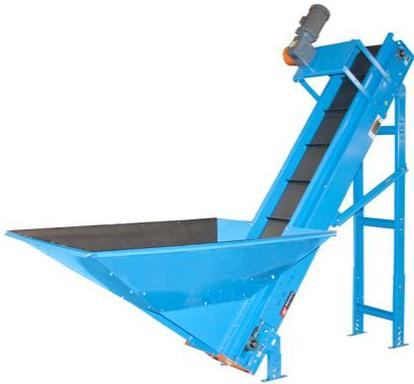
A UHMW lined hopper has been attached to a PC conveyor to handle small parts that are easily damaged. This non-marking covering is on all impact surfaces of a metal hopper which helps protect the finish of the parts as they are dumped to be carried up a 54 degree incline conveyor. This PC conveyor has a #533 black trackmate belt with 1-1/2" molded cleats to move the parts to a line where they are packaged and shipped to the customer.
