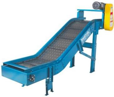
**SteelTrak™** Hinged Steel Belt Conveyors are used to convey virtually any type of metal scrap. These rugged, heavy-duty conveyors are designed for long-term, low-maintenance operations in industrial, scrap, steel chip, and fastener applications. They are ideally suited for carrying hot, oily parts from punch presses, forging machines, etc. to drums or hoppers. Various apron, side-wing, side-rail, and frame designs are available.
