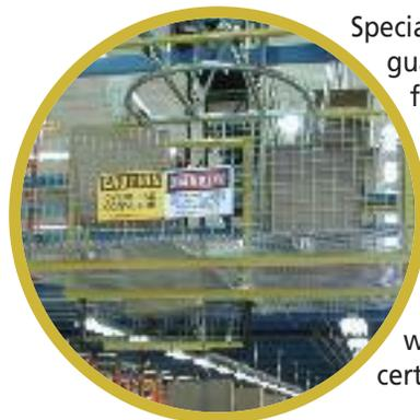
Special protective guarding made from nylon mesh, steel mesh or sheet metal may be added to a system to help ensure worker safety in certain situations.
