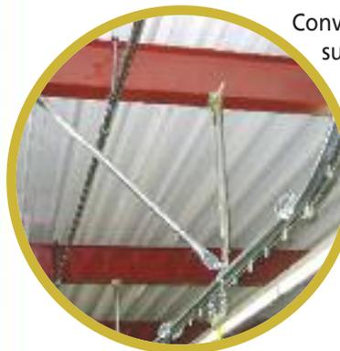
Conveyor can be supported from the ceiling using standard PACLINE components or from any number of custom floor supports.
