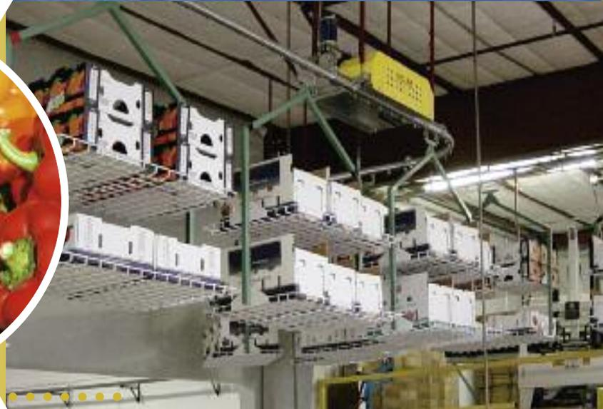
Produce like cherries are highly perishable and need to be packed out quickly and carefully. PACLINE can enhance your current operation by supplying an overhead conveyor that will improve speed and efficiency while maintaining the sanitary conditions required.
