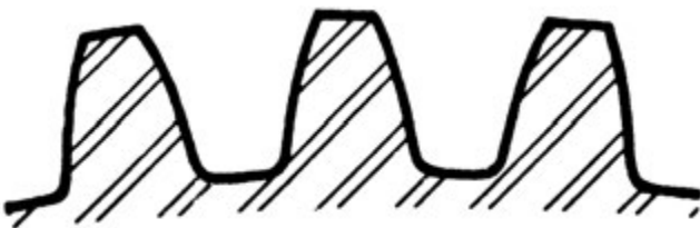
3 Diametral Pitch 1.0472" Circular Pitch
