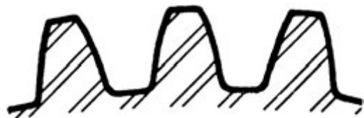
3½ Diametral Pitch .8976" Circular Pitch
