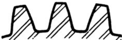
4 Diametral Pitch .7854" Circular Pitch
