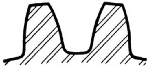
2½ Diametral Pitch 1.2566" Circular Pitch
