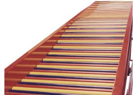
A medium duty gravity roller conveyor features special set high deep side frames with unique hole punching for this roller slide. Gravity rollers include colorful urethane sleeves for protection and smooth ride!
