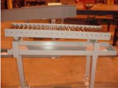
This gravity conveyor is equipped with a grease drip tray and end stops.
