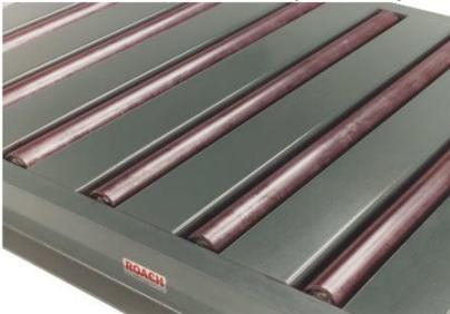
Tread Plates, available in several styles and varying in attachment methods to conveyor frame, are mounted in this gravity conveyor. These tread plates are painted HRS and are welded in place for permanent use.
