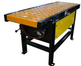
The pan actuates, removing the box from the ball transfer, holding the box in place for filling then disengaging to allow workers to easily transfer the boxes onto the main line.
