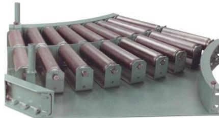
Shown above is a heavy duty Y-switch featuring 297S rollers (2-9/16" diameter, 7 ga.) mounted in a structural frame. Notice the pinned, common shafts in lieu of springloaded rollers.
