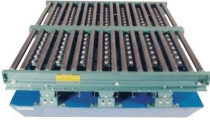
Special Design features strands of ball transfer in which are pneumatically actuated to raise and transfer product. This design also allows product to be rotated as dictated by application while transfer arms are in raised position.
