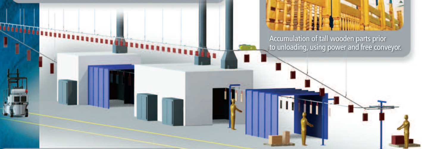
Paint line conveyor moves kitchen cabinets into warmer, unused overhead space for shorter drying time.
