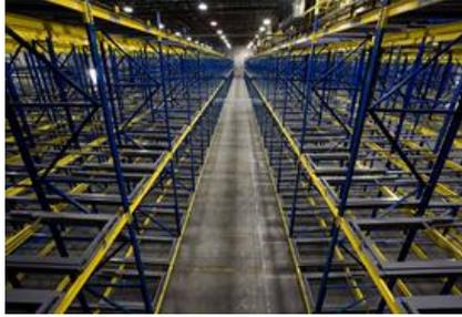
Pushback racking is a pallet storage method that allows pallets to be stored from 2 to 6 deep on either side of an aisle, thereby giving you higher storage density than other forms of racking. A pushback rack system can double or triple your storage when compared to standard pallet rack or double deep racking systems.
