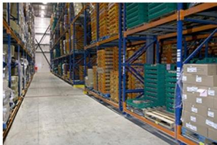
Because the pallets come to the aisle, pushback is much faster to load and unload than any comparable drive-in rack. Additionally, stock rotation and occupancy are greatly improved because each level can store a different product in pushback. Finally, rack damage is significantly reduced because the operator does not have to drive in to the rack to remove pallets.
