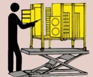
Moving heavy assemblies easily onto a lift
