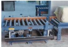
Heavy duty chain driven live roller conveyor runs on a floor-mounted track from foreground conveyor to discharge conveyor shown. Transfer cart is powered to run on track to discharge position where product is discharged from conveyor. Note Roach blue powder paint. Foreground and discharge conveyors are heavy duty, model 3509CDA, chain driven accumulators, handling bales weighing up to 750lbs.
