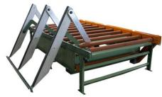
The EZE - Reach Lift Table extends product up and over the side of the conveyor for the operator to work on, then places the product back onto the CDLR conveyor. Rollers are polyurethane-coated and the product rests are UHMW-lined to prevent product marking.
