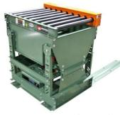
The Powered Transfer Cart is mounted at the end of two conveyor lines. Product is transferred from one conveyor to the other. V-Groove casters travel along the 6' inverted-angle track. Fixtures will be mounted to lifting plates between the rollers to raise and lower product on and off the transfer.
