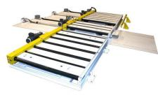
The Heavy Duty pneumatic shuttle cart enables the transfer of product between conveyor lines. The dual stage cylinders hold and pull the conveyor into position.
