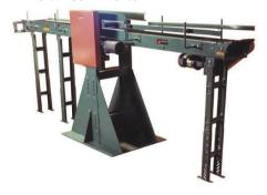
Wheels enter this inverter at infeed of belt conveyor, wheel is inverted 180 degrees and is conveyed to discharge of belt conveyor and on to next process in wheel manufacturing/packaging process. A separate drive (electric) is utilized for both belt conveyor and inverter mechanism. The belt conveyor is model 500BSB with 8" wide belting and B-section V-belt attached to back side of belt for tracking. Rate on conveyor is 5 wheels per minute.
