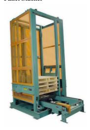
A pallet stacker is shown above designed and manufactured by Roach to stack 48" wide x 40" long x 6" tall pallets. A 2-strand chain drag conveyor, 36" strand centerline is mounted at 17-1/2" elevation which conveys individual pallets into the stacker and stacks of pallets OUT of the stacker.
