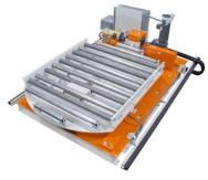
The Low Profile IPT is a transfer cart topped with a powered roller conveyor turntable in a compact elevation. Used to move and rotate large products. The powered rollers assist in the transfer on and off of the turntable. The rollers feature pneumatic roller stops to prevent roller and product movement during cart motion. Also features safety-stop bumpers in case of path blockage while the cart is in motion.
