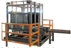
Stack of plywood enters chain drag conveyor and stack is squared when it is fully conveyed into the de-stacker. The chain drag conveyor--actually, a 2-strand chain transfer--is lowered one step and a pneumatically actuated mechanism moves into stack of plywood, clamps and holds entire stack EXCEPT for one sheet. Next, the chain conveyor is lowered to its lowest stage and the individual sheet of plywood exits de-stacker. Process repeats.
