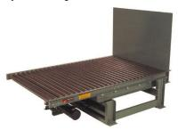
This hydraulic upender features a gravity roller conveyor mounted to bed assembly, model 196S-51-3-H-7, with 36" high end stop. Elevation is 20"TOR. Sized for total live load of 500 pounds, this upender can be activated to move product to its "up" position for testing or assembly operations. Finally, the product may be moved off of the upender tray or lowered to its original position and conveyed off of the gravity conveyor section.
