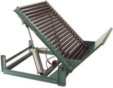
This pneumatic upender features a gravity roller conveyor bed. Product may enter or exit this conveyor on its gravity roller conveyor bed. The upender can be activated to move product to its "up" position for testing or assembly operations. Finally, the product may be moved off of the upender tray or lowered to its original position and conveyed off of the gravity conveyor section.
