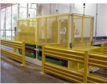
This transfer cart was built to service multiple lines where pallets were feeding off of conveyor systems where the product was being produced. This model is a heavy duty model and was rated for 12,000#.
