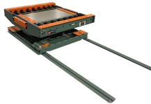
This Low Profile Transfer Cart receives product racks at a low elevation of 9" for easier manual loading of the racks. It then travels to the receiving conveyor, elevates to 19" via scissor-lift, and transfers the loaded racks onto conveyor. The conveyor and transfer cart are powered by MDR (Motorized Drive Rollers).
