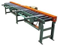
The Bowtie conveyor is designed to convey pipe and other cylindrically shaped products. The trough shape of the roller allows the product to be conveyed with very little side-to-side movement. Angled lifting bars covered with UHMW wearstrip are raised so the rods will roll onto a decline table
