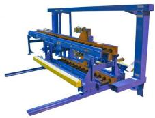
2-tier 251CDLR Transfer Cart. Features pneumatic blade stops and "z" bracket guards for securing product during transfer. Cart is pushed along track via a pneumatic piston.
