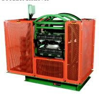
Allows product to enter at one side of conveyor and after "flipping" product 180 degrees, conveys product through unit for next stage in manufacturing process.
