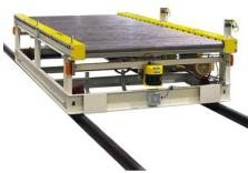
Transfer cars are used in conjunction with our conveying equipment. A typical application utilizes a conveyor deck that is attached to a mobile base. Transfer cars can traverse automatically under the control of a PLC or can be used in a hand-push application and/or lean manufacturing operations.
