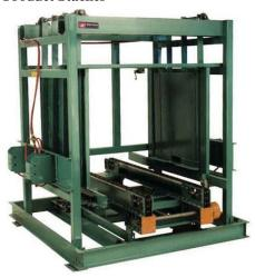
When product enters chain drag conveyor, side mounted mechanism moves into product, clamps it and raises product for clearance to allow next product to enter. Once second product has moved into place on the chain drag conveyor, first product is lowered onto second product and both are raised to allow additional products to enter conveyor. Process repeats.
