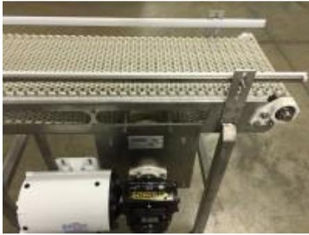
This Stainless Steel Plastic Belt Conveyor was built to conveyor frozen foods without damaging the packaging and product. The UHMW guides keep the product in route without rubbing the product labels off the container.
