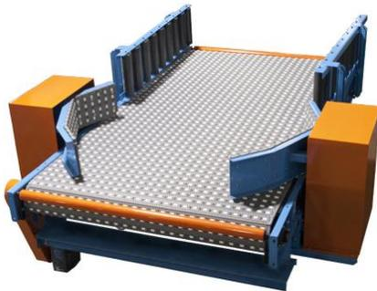
The tire centering device will align tires in the center of the conveyor to be unloaded by robot. As tires move into the centering area the paddles clamp onto the tire placing it in the center. The 52" wide series 400 roller top belt allows the conveyor to operate continuously while the tire is clamped in place. Roller top belt has also been attached to the face of the paddles to aid in alignment.
