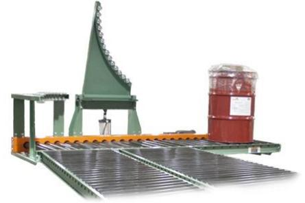
90° dual-lane barrel diverter features specially curved diverter arm mounted with skate wheels to allow smooth diversion of barrel products. A pneumatic arm lifts the first diverter to allow passage of barrels to the second diverter.
