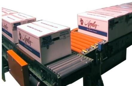
The pneumatic indexer creates specific spacing between products. The 18" long pneumatic operated indexing conveyor is located at the discharge end of the line and has a cylinder that raises and lowers at specific intervals and prevents product stacking and adds gaps onto the next conveyer line.
