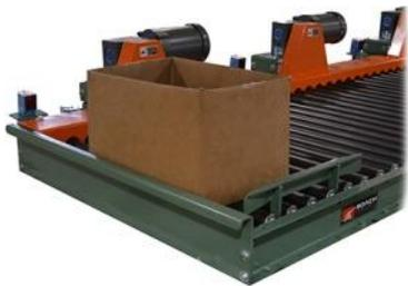
A Puller arm is mounted at the discharge end of the conveyor to position product for a robot to pick up. A photoeye senses that product is in the zone activating the puller arm to move the product to the drive side. A pressure switch is incorporated to accommodate multiple product sizes. Once positioned the puller arm then resets for the next product.
