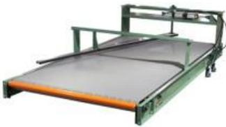
This 54" wide plastic belt conveyor has a 3 position pneumatic diverter mounted onto it for diverting 25lb bags. The diverter arm moves the bags to the center or 30 degrees to the left or right to be transferred onto conveyor at the discharge end. The 54" wide series 900 flush grid grey polypropylene belt allows the bags to easily move with the diverter arm.
