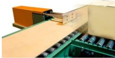
The Primo Sort High Speed Sorter was designed in response to an increasing demand for high speed distribution equipment. Up to 75 sorts per minute (based on size of product) can be economically and accurately sorted with the Primo.
