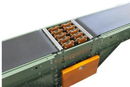
The 796 Sort Belt Pivoting Belt Diverter has a high rate of package sortation. As many as 75 cartons may be accurately sorted per minute with belt speeds as high as 300 fpm. Guards removed to show chains; do not operate with guards removed.
