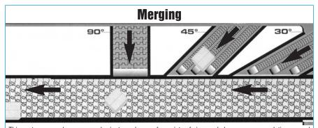
This system properly merges and orients packages of a variety of sizes and shapes, accommodating several infeed lanes from a variety of merge angles. The spinning rollers direct the products to the conveyor edge.
