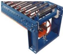
This is a specially designed stop for mounting in Roach 196LS line shaft driven conveyor. A pneumatic cylinder moves the roller stop assembly upward UHMW channel when activated.
