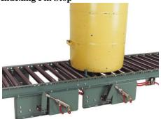
Modified pneumatic stops are used together to index product. In this instance, a barrel container is indexed with two modified package stops, model PRSG. When offloading, stop nearest discharge end of conveyor is lowered while stop nearest infeed of conveyor is raised. Product is released by stop in lowered position while product is held by stop in raised position.
