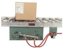
This is a pneumatic roller stop designed for Roach light duty gravity conveyor, model 138G / 138A.
