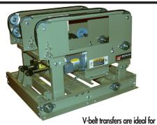
medium duty applications and are often used where product could be damaged by strands of chain on heavier duty chain transfers. Unit at left shown with frame cutout for use in belt driven live roller conveyor with 6" wide belting.
