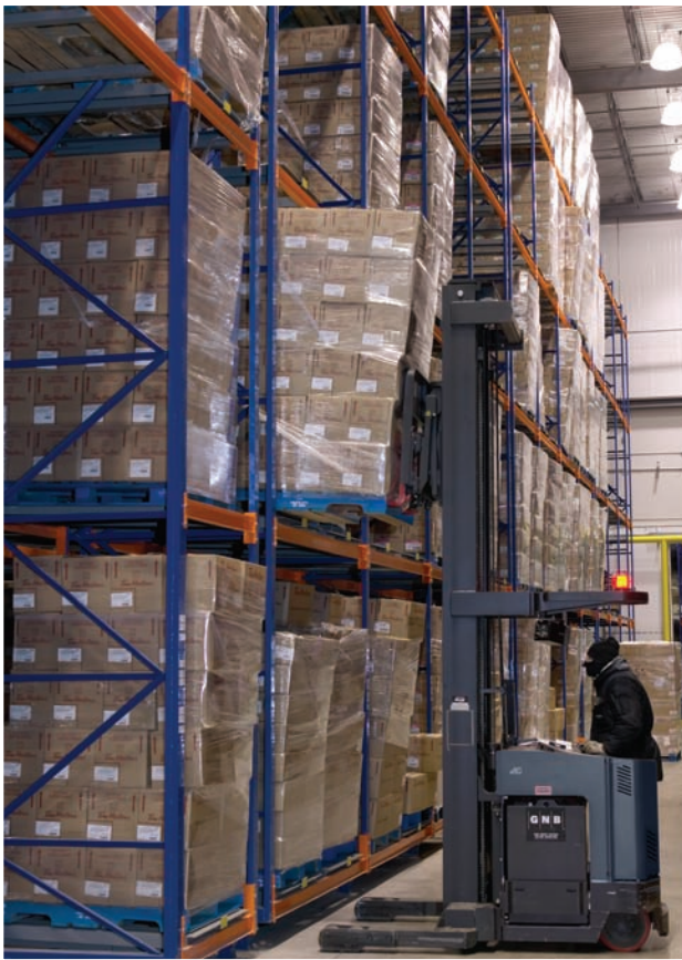
▲ 4-deep, 5-high pushback application in freezer
