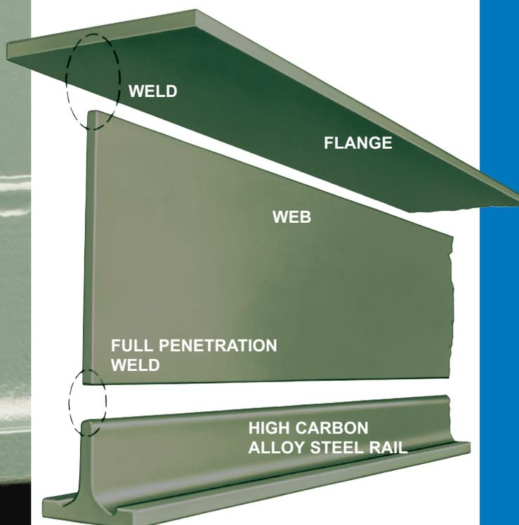
Tarca® Track has a mild steel top flange and web and a high carbon steel lower rail with raised tread to resist peening.
