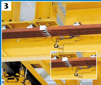
3. The rollers make contact with the wedge and self-align within 1-1/4" horizontal range. As both beams are interlocked, forks on powered and non-powered beams are raised for free passage of carrier (see Photo 3).
