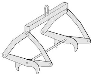
This **Dual Gripping Tong** system will support and stabilize longer, larger loads that can sustain the force of the entire load on a smaller surface area. When the narrow gripping arms engage the item, significant pressure will be applied. Ideal for handling bundles of steel that are round in shape.
