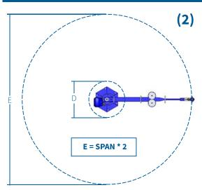
\*\*Units with 10' spans must be mounted to an 8" reinforced concrete floor based on 3000 psi concrete pressure and soil pressure of 2500 psf
