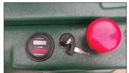
Hour meter, battery status indicator, charger controls and emergency e-stop
