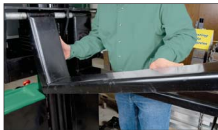
Forks on straddle models are adjustable from 12" to 27" wide
