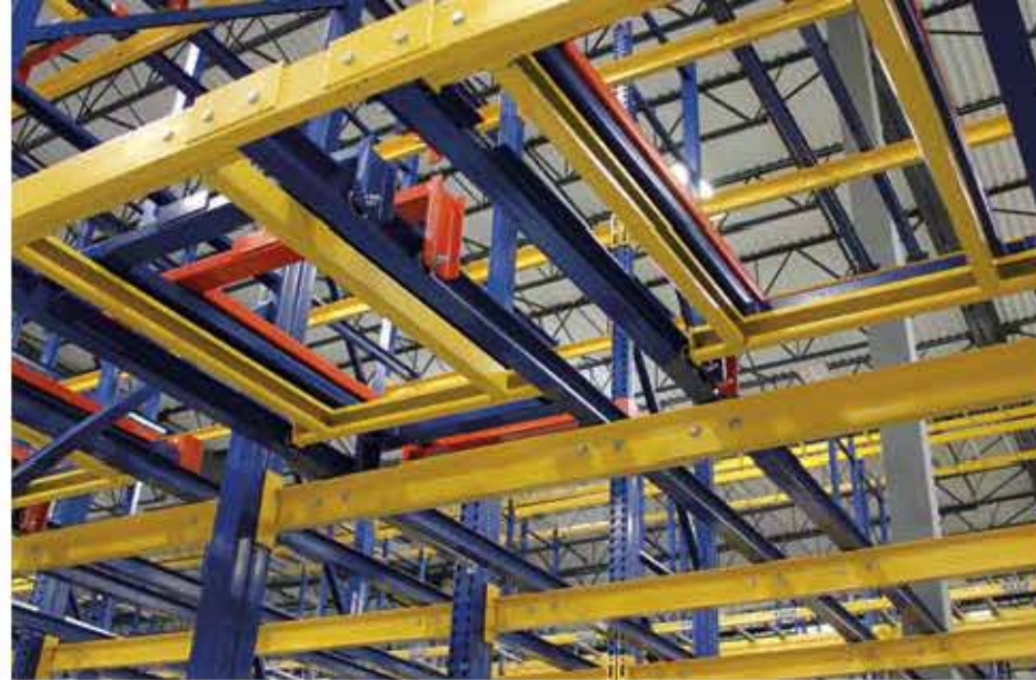
Colored carts let drivers identify pallet positions to help place and retrieve pallets in the system.
