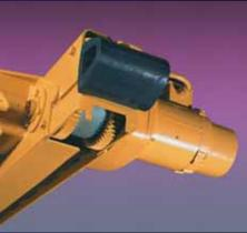
Two driven wheels are used to propel the trolley. The trolley traverse is driven by a TENV motor with a standard AC disk brake. This drives a geared flange, fixed axle wheel with a secondary pinion line shaft connected to a drive pinion in the other end truck.
