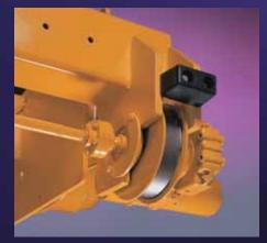
Totally enclosed, heavy-duty oil bath lubricated trolley traverse drive turns two rotating axle wheels connected by a line shaft. All wheels are supported on both sides by anti-friction bearings.
