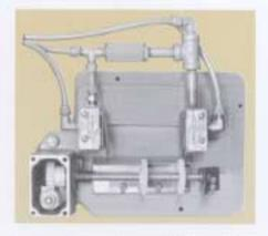
A geared traveling nut limit switch is standard. It is a two position switch with adjustable upper and lower limits and is designed to prevent accidental hook over-travel.
