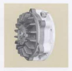
The disc type motor brake controls hook drift and facilitates load spotting. This spring-engaged brake is designed to operate if the air supply is interrupted for any reason. The motor brake is self-adjusting and incorporates cooling fins to dissipate heat. It is enclosed against dirt, water, and oil and is designed to independently hold the full rated capacity of the hoist.
