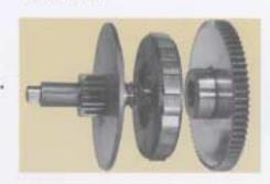
The load brake on Yale Cable King hoists is a self-actuating, Weston screw-and-disc type brake. It is mounted in the gearbox between the first and second gear reductions, and operated in a continuous oil bath to help dissipate heat. The brake is self adjusting and operates whether the power is on or off. The load brake is capable of safely holding the rated capacity of the hoist.
