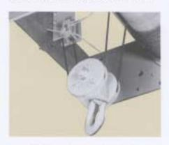
An additional upper limit switch is standard as a backup and is designed to prevent hook over-travel in the "up" mode. It is activated by the bottom block.
