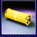
Machined Rope Drum Large diameter welded construction — deep grooved and precision machined to give maximum rope life. Pictured is a right and left hand grooved true vertical lift drum.
