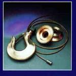
**Spark Resistant Features** Bronze and high bronze alloys incorporated in key components such as hooks, lower blocks and wheels, along with stainless steel wire rope, help prevent incidental sparking in hazardous locations.
