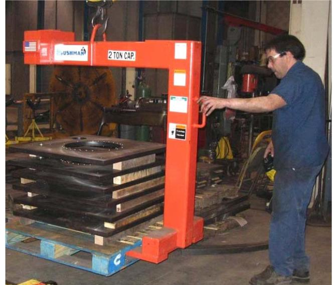
Bushman pallet lifters are available in capacities from 500 pounds to 20 tons. Pallet lifter features include:
