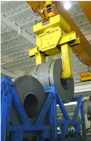
Coil grab features include motorized or manual adjustment, low headroom designs, replaceable wear bars for high duty cycle operation, optical sensors, full length coil sensing flapper assemblies on drop legs, protective padding and rollers, special bail configurations, motorized rotation and built-in weigh scales.
