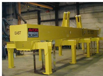
Sheet lifters feature hand wheels, chain wheels and motorized leg travel. They can be equipped with low profile designs; end hooks; load weighing systems; and self-locking leg designs that prevent opening under load.
