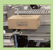
More than 100 weight readings are taken, then averaged, as a box speeds over the scale.
