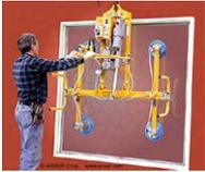
**Typical Vacuum Lifters with powered tilt (powered upenders) for handling your tilting needs with ease. Powered tilting action is designed to be stopped at any intermediate angle by one person.**
