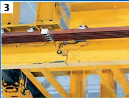
3. The rollers make contact with the wedge and self-align within 1-1/4" horizontal range. As both beams are interlocked, forks on powered and non-powered beams are raised for free passage of carrier (see Photo 3).
