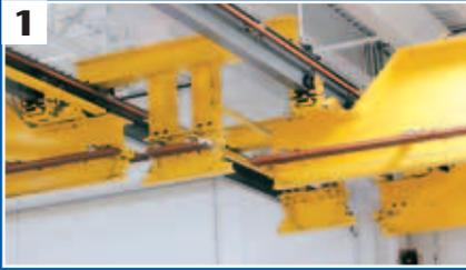
1. Both bridge girders approach the crossover track. The operator pushes a button powering a gear motor that activates a pair of rollers (see Photo 1).
