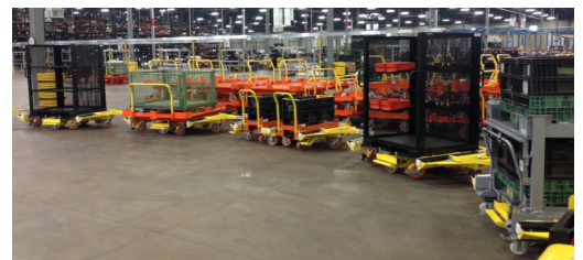
CarryMore® Tugger Cart System in use on the line.
