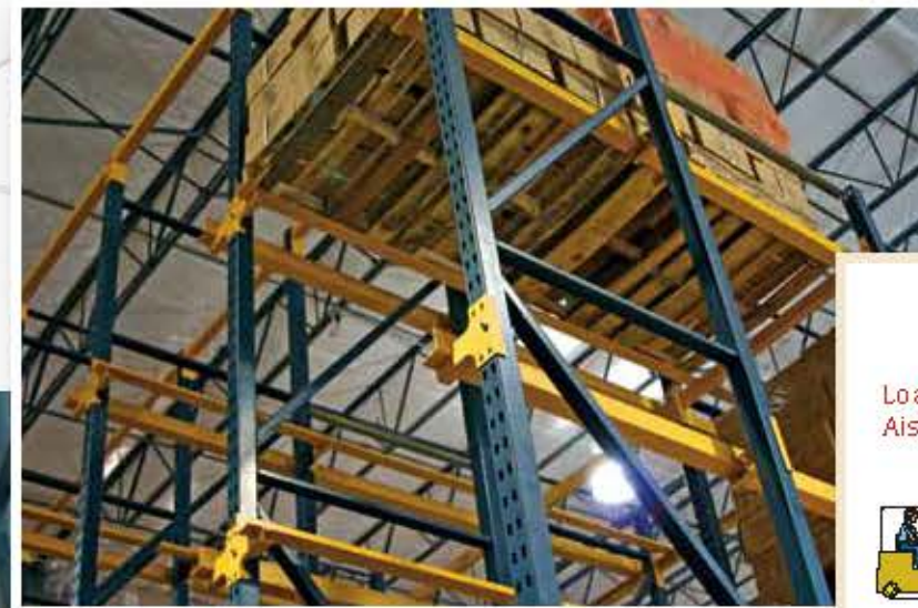
Pallets rest on rails within the bay.
