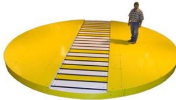
This turntable was designed to rotate a 3500 lbs. product while workers are present. The 251 CDLR has a 5' conveying surface with treadplates mounted between the rollers. These treadplates are alternating colors yellow and white on each end of the conveyor to help the operator center the product before rotating. The heavy duty center pivot turntable is a 22'8" in diameter with casters to support the outer ring.
