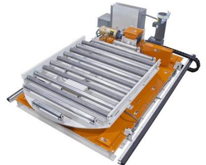
The Low Profile IPT is a transfer cart topped with a powered roller conveyor turntable in a compact elevation. Used to move and rotate large products. The powered rollers assist in the transfer on and off of the turntable. The rollers feature pneumatic roller stops to prevent roller and product movement during cart motion. Also features safety-stop bumpers in case of path blockage while the cart is in motion.
