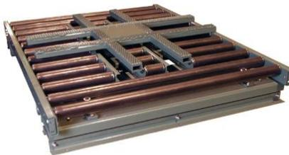
This grid turntable was designed for low elevations. The product is manually positioned and centered above the grid. The conveyor is then lowered leaving the product sitting on top of the grid turntable. The turntable is then rotated 90 degrees and the conveyor is raised to pick the product up. The product can now be manually discharged.
