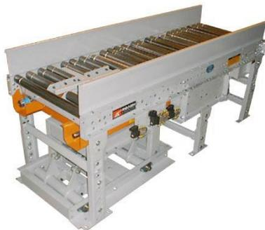
A cross type pneumatically actuated turntable is mounted in this line shaft driven conveyor (foreground) to re-orient position of product. This turntable rotates 16" wide x 20" long x 25 lb. product 90°.
