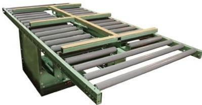
This Grid Turntable is mounted in a 196 gravity conveyor with 3/16" thick gray PVC covering on the tread rollers. The grid arms are covered with non-marking belt which compliment the PVC covered rollers to avoid damaging the finish of the product. The grid is pneumatically raised and can be manually turned 180 degrees by the operator.
