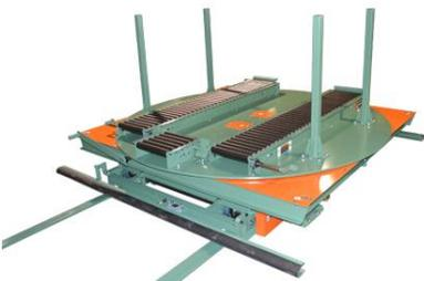
This is a manually operated turntable combined with a transfer cart. Automotive parts on a pallet are conveyed onto the turntable. This turntable has 2-199S gravity conveyors spaced apart to give an effective 50" BF. To contain the product these gravity units have heavy duty butt end stops at the discharge end and dual blade stops at the infeed end. The operator can release the lock for the turntable and use the 4 post to manually rotate the product for inspection.
