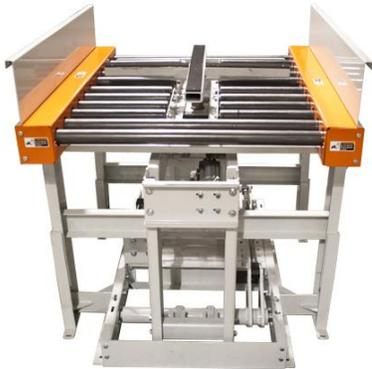
This cross turntable is mounted in a 192CDLR to handle a product weighing 110 lbs. Once the product is in place the cross turntable is pneumatically raised and rotated 180 degrees to change the product's leading edge.
