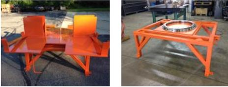
This heavy duty manual turntable was a custom built unit. This turntable featured 2 - 180 degree stops with foot release levers. Each side was built to handle 6000# with an empty load on the opposite side.
