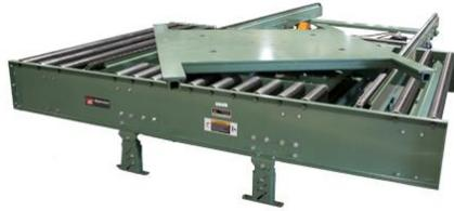
CT 280 Chain Transfer moves product onto the turntable. The turntable is raised pneumatically via operator input and can then be turned manually to rotate the product.
