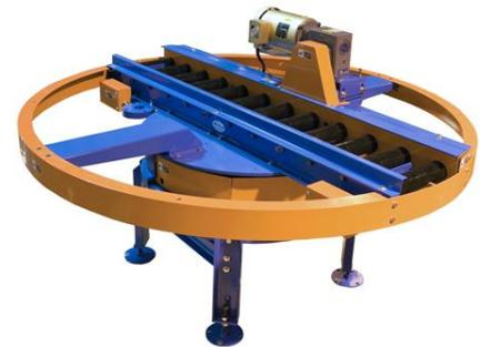
IPT mounted with a 251CDLR. Pneumatic blade stops halt product on the CDLR while the IPT rotates the product. IPT is on raised structural supports for mounting above a second line.
