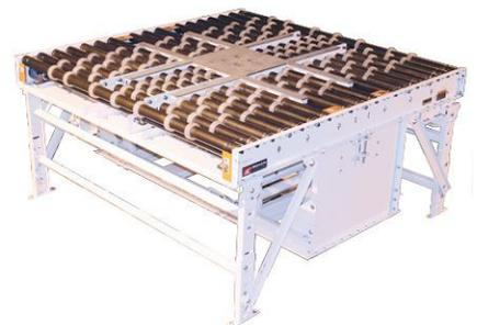
Polyurethane bands are located on rollers to provide minimal points of contact on the glass panels and reduce the chance of breakage or scarring. Features a central pop-up ball turntable for repositioning glass panels.
