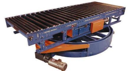
This heavy duty indexing turntable includes model 251CALR live roller conveyor stationed as the transfer device. Here, plywood slip sheets loaded with varying weights, sizes and styles of sheared steel product are transferred via this heavy duty indexing turntable. Product moves to perpendicular conveyor lines via this conveyor eliminating wasted floor space resulting when large-radius tapered roller chain driven live roller curves are used.
