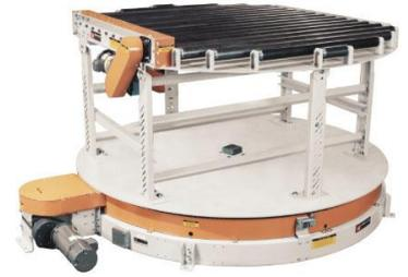
This heavy duty indexing turntable includes model 251CDLR chain driven live roller conveyor stationed as the transfer device. Product is transferred to perpendicular conveyor lines via this conveyor eliminating wasted floor space resulting when large-radius tapered roller chain driven live roller curves are used.
