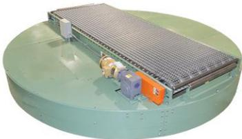
An 11' long wire mesh belt conveyor is mounted on a heavy duty center pivot turntable. The product is castings on a wood pallet weighing up to 3000 lbs. The wire mesh belt was used to handle the extreme temperatures and dirty environment.
