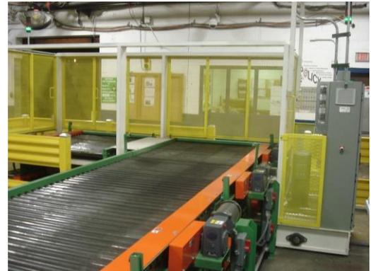
This transfer cart is equipped with an Over/Under Conveyor system that feeds the bottom of each conveyor line with empty pallets while at the same time accepting the two full pallets on top.
