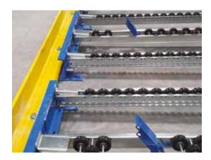
Layer picking uses specialized material handling equipment to select multiple cases, or the entire carton layer, at one time, thus increasing pick rates reducing manual labor costs. Mallard's LP-400 Pallet Separator is used within the layer pick pallet flow system to separate the front pallet until all cases are selected, allowing safe manual removal of the empty pallet.
