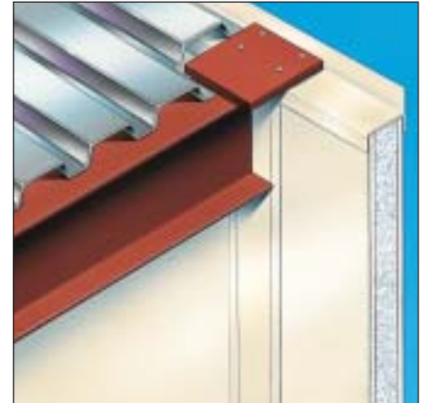
Loadbearing roof beam.
