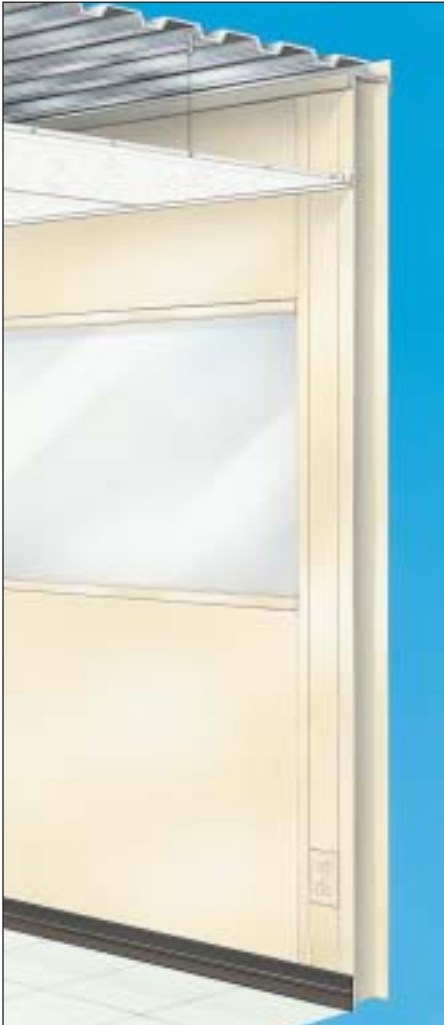
Ceiling suspended from roof deck.
