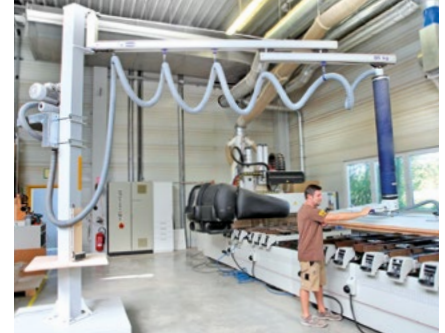
Telescopic jib for confined working areas
