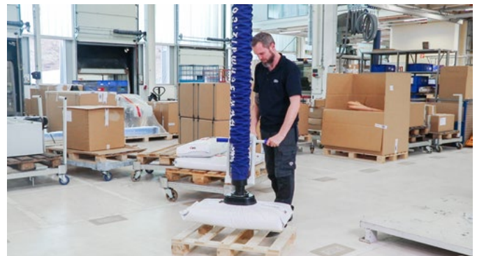
JumboFlex High-Stack when handling bags
