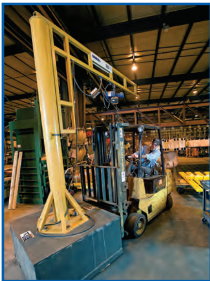
Freestanding Workstation Jib Crane with Portable Base
