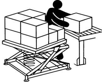
Work station applications to load or unload pallets represent one of the most common and most popular applications.
