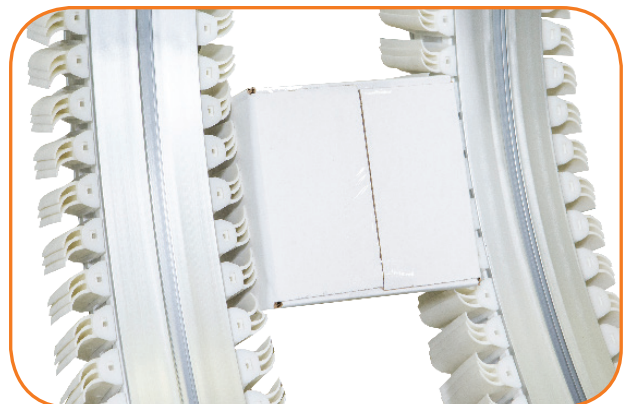
Products are wedged between opposing conveyors
