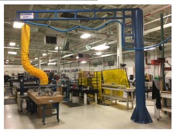
between 85-100 lbs and range up to 30" wide x 84" long. The oversized arm on the lifting device keeps the operator at a comfortable distance from the box, not having to lean over or across to pick and place. The long span on the workstation crane allows the operator to have multiple pallets in place to stack product on.
