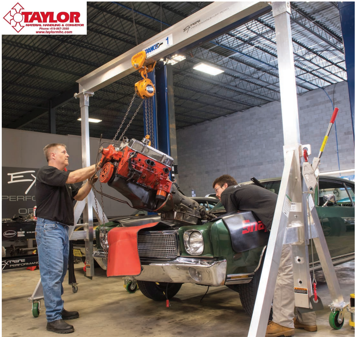
A-Series Aluminum Gantry Crane. Optional height adjustment with Lug-All® cable hoists.
