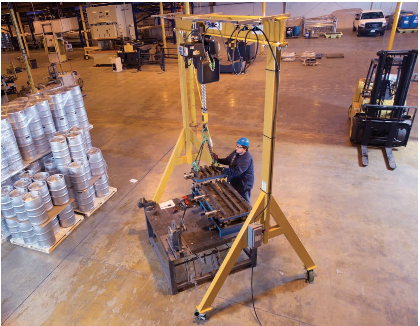
A-Series Fixed Height Gantry Crane
